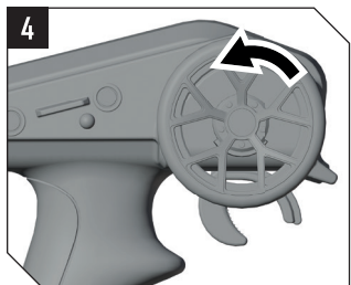
4 Go to Full Left Steering on the transmitter. Blue LED on ESC will flash once and wheels will turn to the left.
